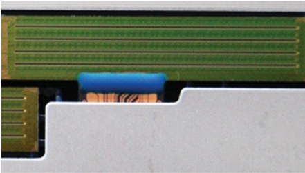
Figure 5: Detail of an HP Thermal Inkjet die
